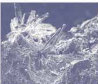
Asbestos Fibres on a Broken AC Sheet. SEM magnification 200x (Dyczek, 2004:8).
